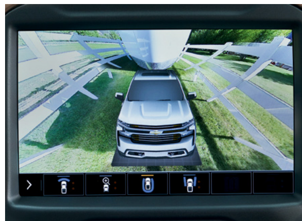
Bowl View Provides a rear-facing 3-D surround view, useful for low-speed backing manoeuvres.
