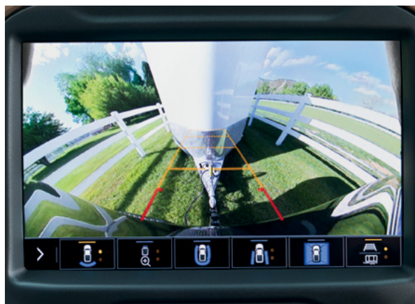
Rear Camera View Displays rear view to assist with parking and tight manoeuvres.
